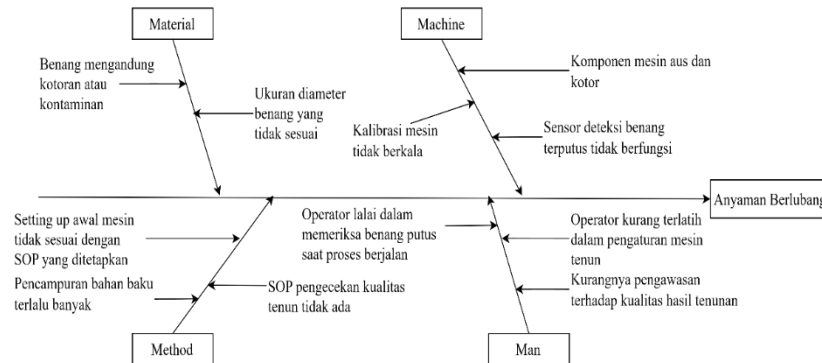
Figure 5. Fishbone diagram root of the problem of perforated weaving defects
