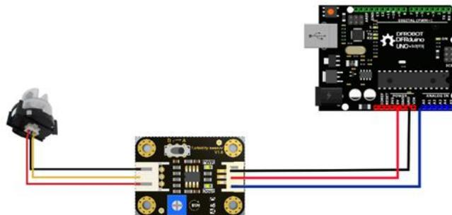
**Figure 2.** Installation of a Turbidity sensor to measure TDS levels in water.
