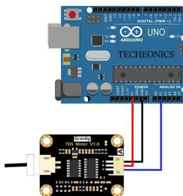
**Figure 1.** Installation of a TDS sensor to measure TDS levels in water.
